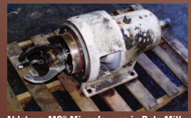
Ahlstrom MC ® Mixer for use in Pulp Mill
