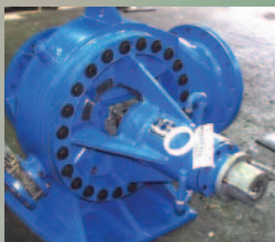
Impco 600 High Shear Mixer Use: Bleach Plant (SS, Hast C, or Titanium)
