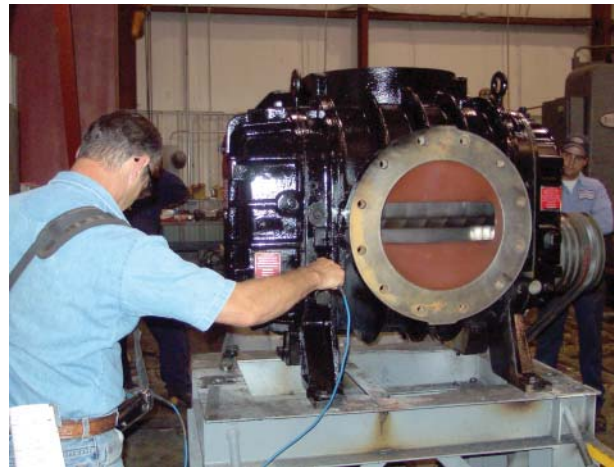
Testing a rebuilt blower.
