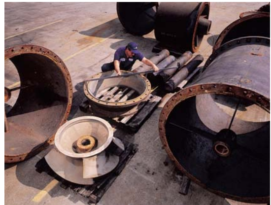
Disassembled pumps are inspected for unusual wear.
