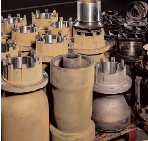
Special vertical applications welcomed. Above are some geothermal units that are being rebowled. ITT Industries can handle some of the toughest applications.
