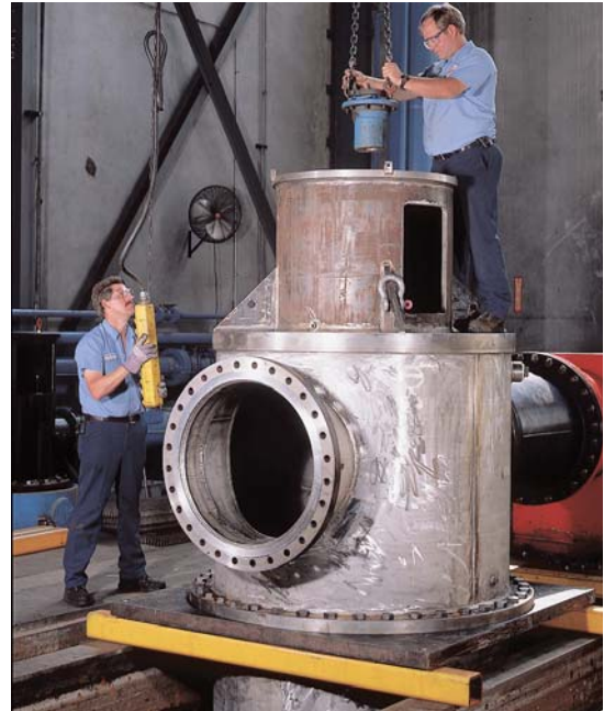
New discharge heads can be provided to address vibration problems. Complete head analysis can be accomplished if required and tested at our Los Angeles facility.
