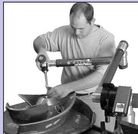
Figure 1, Scanning part using CMM
