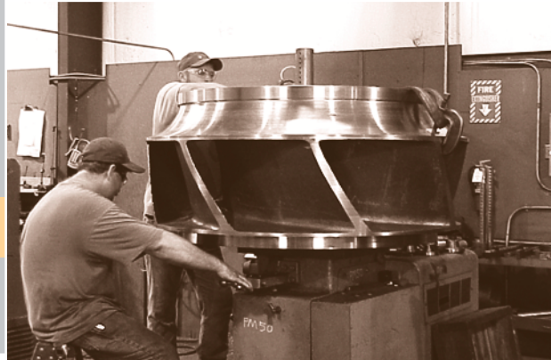
Impeller being keyed during the machining phase.
