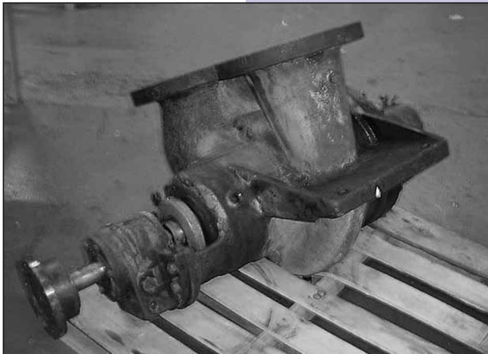
Extensive repair and upgrade were required on this API unit.
