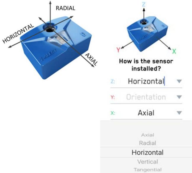
The axis can be changed from the App to account for different installations. It is as easy as following the steps once the sensor is discovered and choosing the desired axis as shown below.
