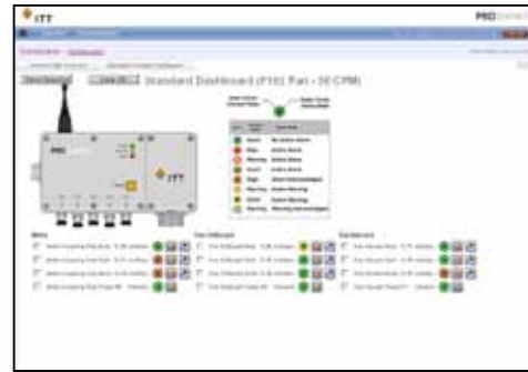
The standard ProNet dashboard includes an interactive interface for every Data Monitor.
