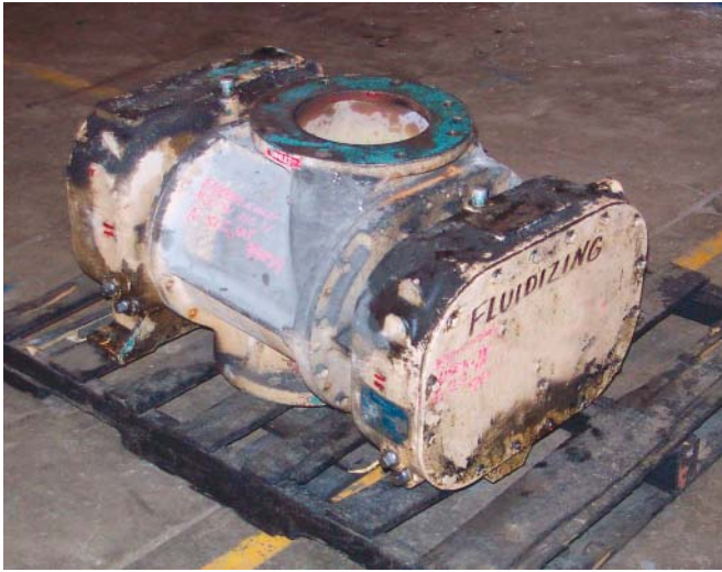
(Before) Ash blower ready for tear down and inspection.
