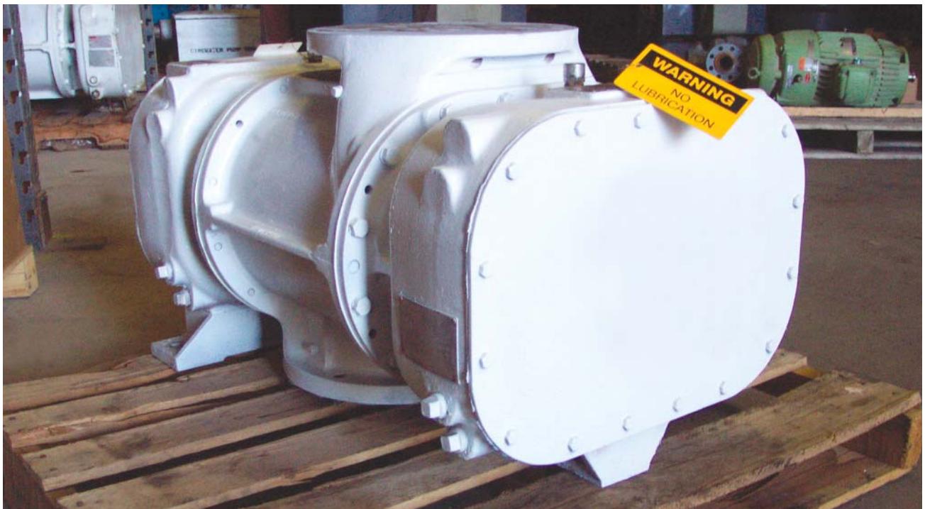
(After) Ash blower rebuilt, tested, and ready for delivery.
