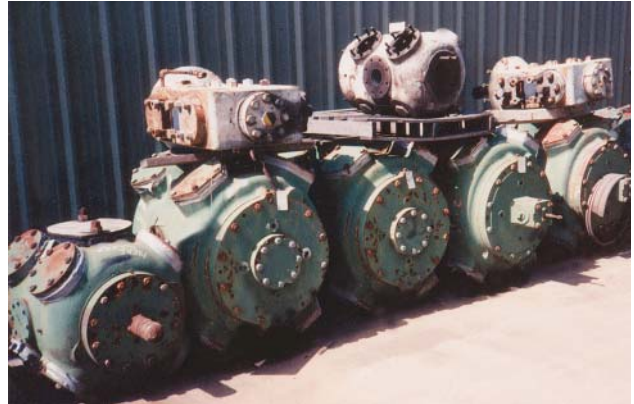
Compressor cylinders to be repaired.
