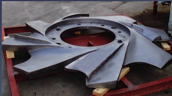
Pulper Impeller for use in Recycle Area, "High Wear"
