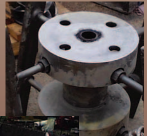
Screen Rotor for Use in Pulp Mill "Repair or New"
