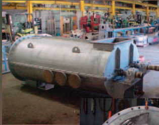
Ahlstrom LRS Pump. Use: 4-6 pumps for every digester. ProCast Makes all Parts.
