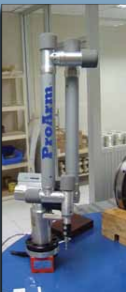
We use CMM Technology to create three dimensional drawings in a digital format.
