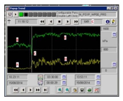
As the flow would decrease (A), the pressure in the system would increase (B). Then as dust suppression cannons would come online (C), the flow demand would sharply increase and the pressure would drop to unacceptable lows. As the cannons switched on and off, the flow and pressure would fluctuate accordingly (D & E).
