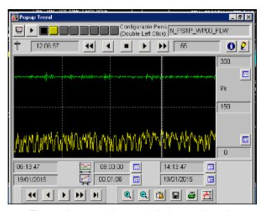
The trend over an 8 hour period shows a dramatic improvement compared to the pressure spikes of >700kPa in the original system.
